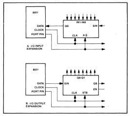
Figure 2.8. I/O Expansion Technique
